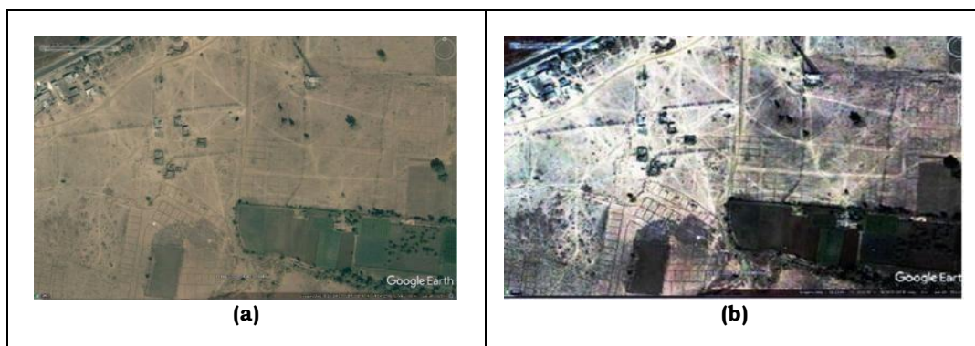
Figure 3. a) Input image of year 2003, b) Result of Histogram Equalization on 2003 image
